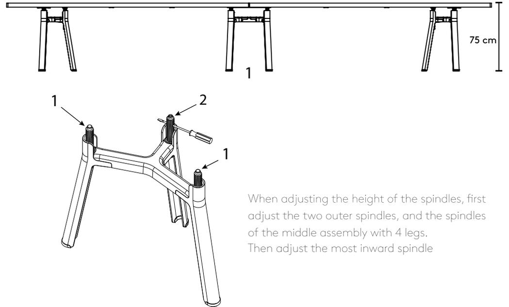
When adjusting the height of the spindles, first adjust the two outer spindles, and the spindles of the middle assembly with 4 legs. Then adjust the most inward spindle
