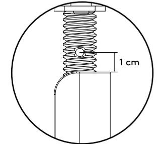
! - Make sure the holes align properly with the provided screws.
