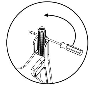
Turn the spindles until the hole is approximately 1cm above the top of the leg
